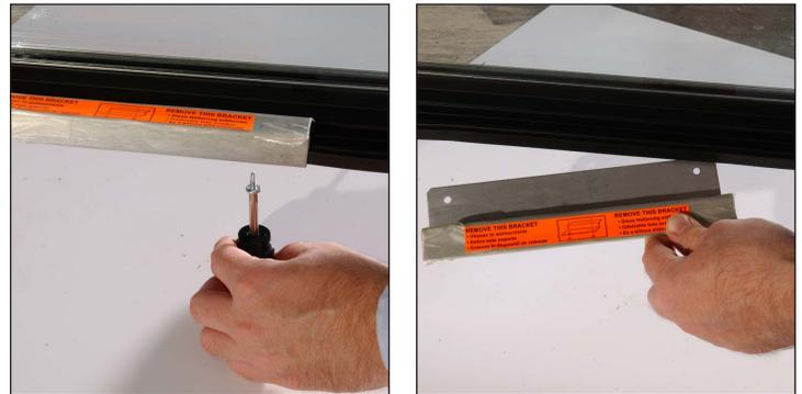
**Fig. 2.** Remove the glass swing door shipping bracket. Do not discard.
