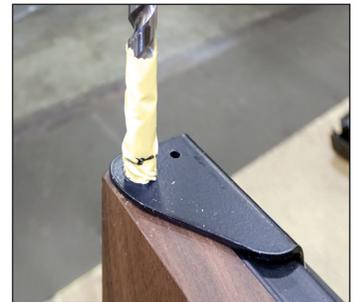
**Fig. 9.** Drill the 3/8" hole first. THEN drill the 17/64" hole.
