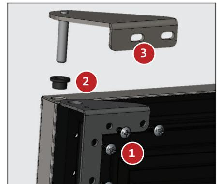
Fig. 7b. Top hinge component assembly.
