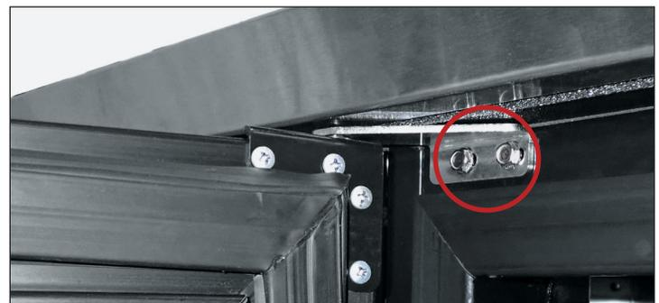
Fig. 4. Carefully remove the door from the unit.
