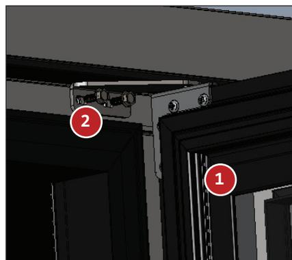
Fig. 10. Install the top hinge and the door.
