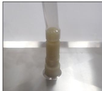
Fig. 5. Hose installed on spill tray tube.
