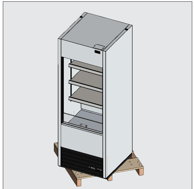
**Fig. 3.** When lifting the appliance, do not use countertops, doors/drawers, or grills as a lifting point.
