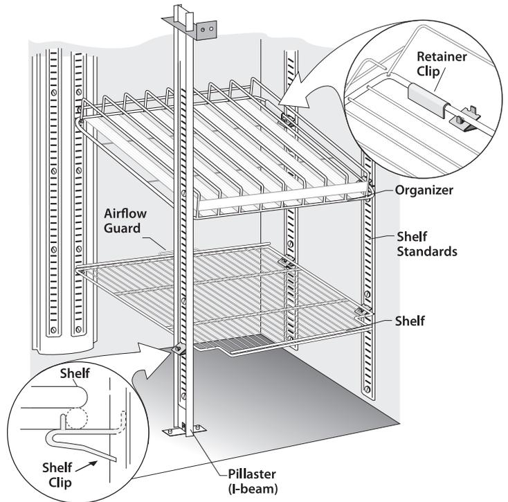
Fig. 5. Installed shelf clip.
