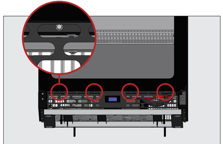
**Fig. 3.** Remove the front grill bolts to access the shipping bolts.
