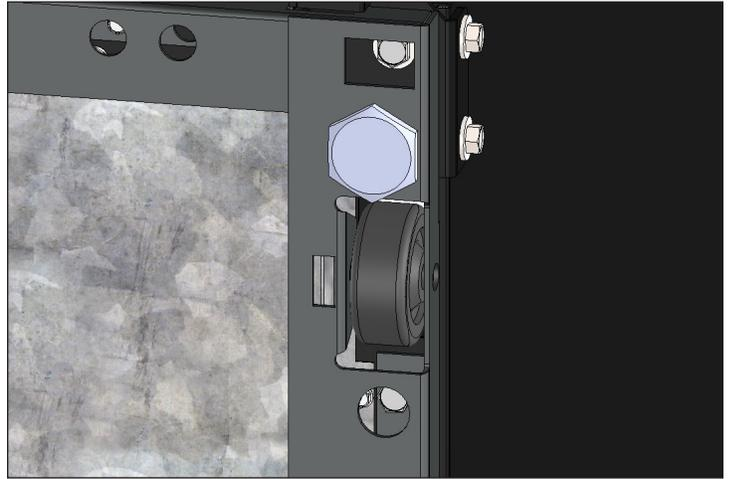
**Fig. 11.** Position the castor.
