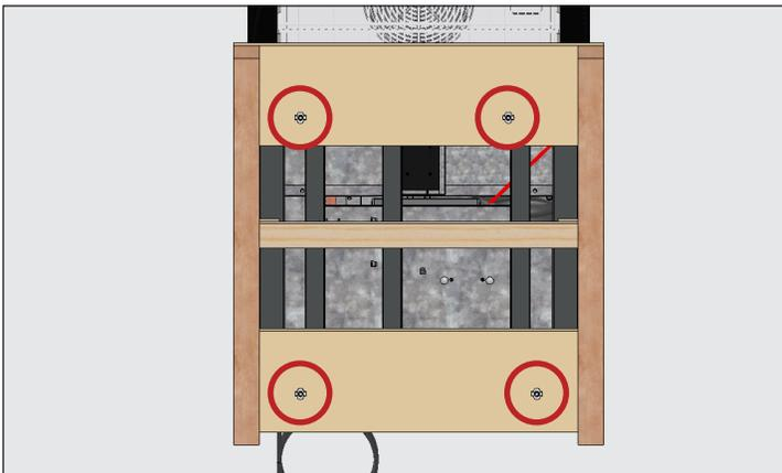
**Fig. 2.** Example of shipping bolt locations.
