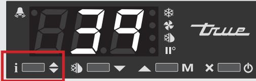
2. While holding info, press the up or down arrows to adjust the setting.
