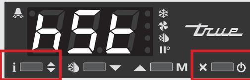
2. Press the up arrow until the display shows **dFt**.
