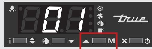
5. Release all buttons and wait for the control to display the current appliance temperature.
