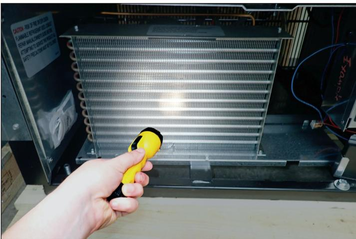
Fig. 3. Verify all blockages have been removed.
