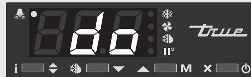
To silence the alarm, shut the door or press **ANY** button on the control. The display will continue to flash **do** until the door closes.
