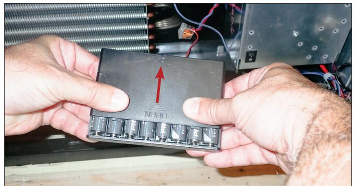
Fig. 4. Slide the battery cover off.
