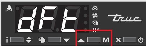
3. Press and hold info until the display shows the current defrost interval time. **DO NOT RELEASE THE BUTTON!**
