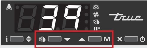
3. Release all buttons and wait for the control to display the current appliance temperature.
