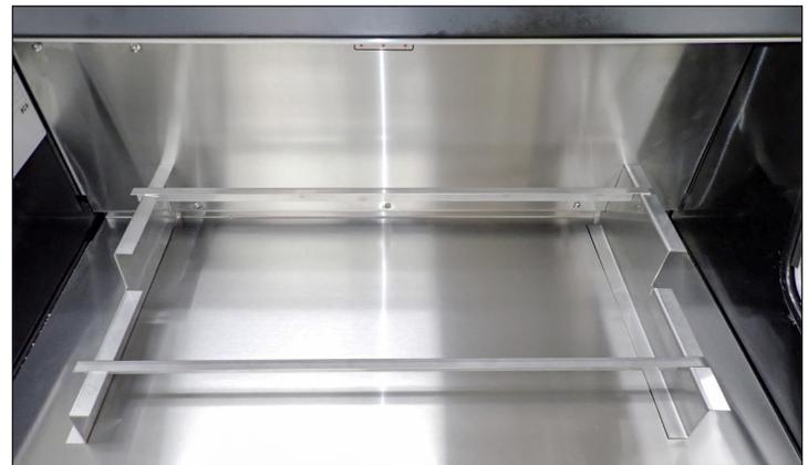
**Fig. 1c.** Installed shelf risers and shelf supports.
