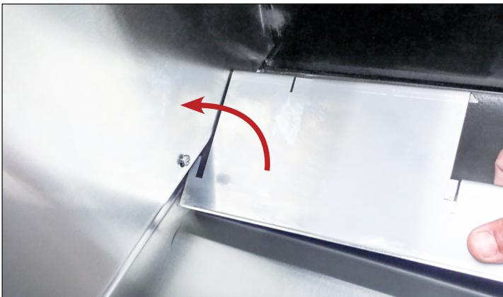
**Fig. 1b.** Carefully slide the risers onto the back wall.
