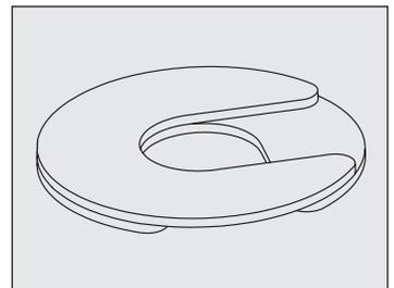
**Fig. 7.** Install multiple shims with offset slots.
