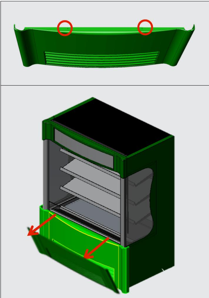
Fig. 3. TAC-48SM: Remove the screws and tilt the top of the grill forward.
