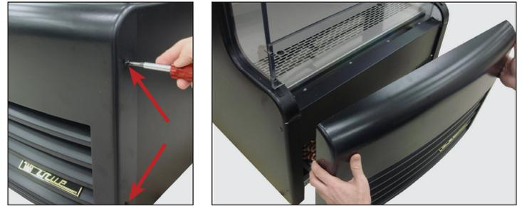
Fig. 2. TAC-14GS-HC-LD Grill removal. Lift grill away from cabinet after removing screws.
