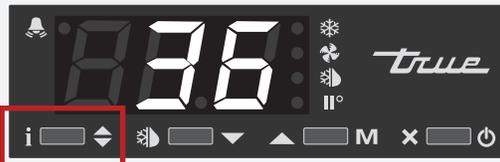
7. Release all buttons and wait for the control to display the current appliance temperature.
