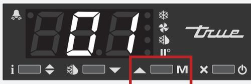
4. Release all buttons and wait for the control display to alternate between **hSt** and **dLY**.
