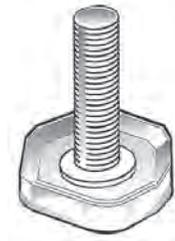
**Fig. 1.** Leveling screw.
