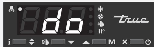
To silence the alarm, shut the door or press **ANY** button on the control. The display will continue to flash **do** until the door closes.
