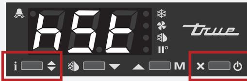
2. Press the up arrow until the display shows **dFt**.
