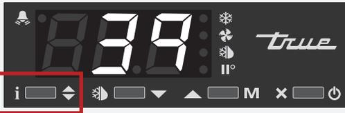
2. While holding info, press the up or down arrows to adjust the setting.
