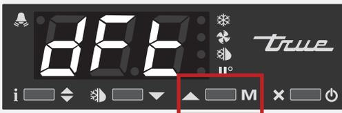
3. Press and hold info until the display shows the current defrost interval time. **DO NOT RELEASE THE BUTTON!**
