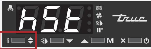
2. Press the down arrow until the display shows **Loc.**
