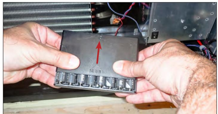
Fig. 4. Slide the battery cover off.
